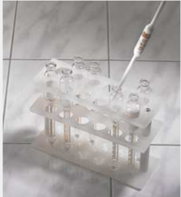
Fig. 2 10.75 ml of milk are pipetted into the butyrometer
